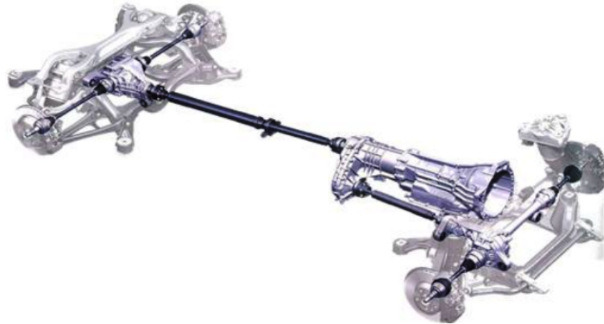
Figure 3-1, Typical IRS AWD Driveline
